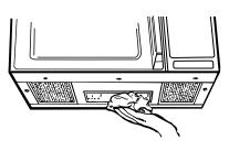
**Clean** off the grease and dust on hood surfaces often. Use a solution of warm water and detergent. About 1 tablespoon of ammonia may be added to the water. Take care not to touch the filters and enamel surfaces with this solution; ammonia will darken metal.
